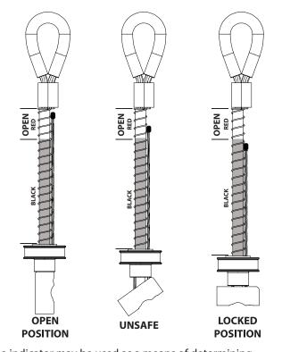
The indicator may be used as a means of determining toggle position when view of toggle bar is obstructed by the anchorage. If indicator is aligned with the red zone, toggle bar is in open or unsafe position. If top of indicator is below the red zone, toggle bar is in locked position.
