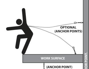
\*The user shall be equipped with a means of limiting the maximum dynamic forces exerted on the user during the arrest of a fall to a maximum of 8 kN (1800-lbf). In the EU these forces must be limited to 6 kN (1350-lbf).
